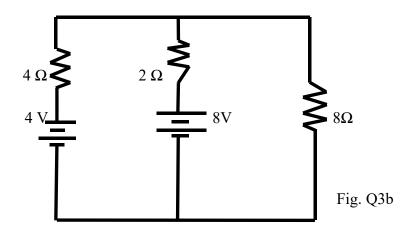
(ii) Hence, determine the power dissipated in the 8  $\Omega$  resistor (12 marks)
