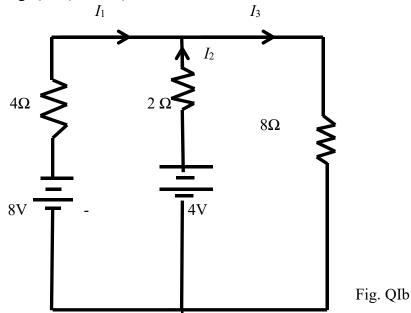
c ii. Convert the network circuit in Frg.Q1c to an equivalent Thevenin's circuit
