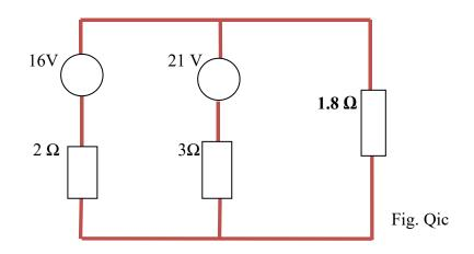
ii) Determine the current flowing in the  $1.8 \Omega$  resistor using Thevenin's theorem or Kirchhoff's theorem (8 marks)
