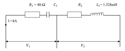
The supply frequency is 2.5kHz and find a sinusoidal expression representing  $V_1 + V_2$
